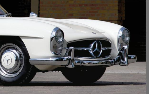
SPECIFICATIONS: 225 bhp (DIN), 250 bhp (SAE), 2,996 cc overhead-cam six-cylinder engine, four-speed all-synchromesh gearbox, independent front suspension with twin wishbones, coil springs and anti-roll bar, single-pivot swing axle rear suspension with compensating spring and coil springs, hydraulic telescopic shock absorbers, and hydraulic front disc, rear drum brakes. Wheelbase: 94.5"
