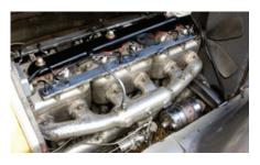
T-head configuration, produced in several sizes; for most of the teen years these were of 38, 48 and 66 horsepower. In 1918 the 38 and 66 were discontinued and the 48 redesigned with dual valves.
