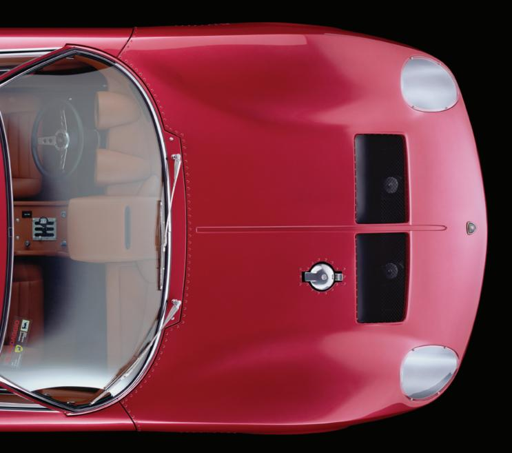
According to Fukuno, the first SVJ was s/n 4860, built from a brand new Miura SV for the President of the Lamborghini dealers in Germany, Hubert Hahne. The exterior characteristics of the Jota were replicated as much as possible: air outlets at rear of fenders, racing fuel filler cap and fixed headlights. The powertrain was changed to 447PS, which was the spare engine for the original Jota, s/n 5084. This car was delivered 29th April, 1971 with production certification SVJ.
