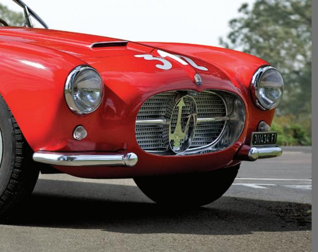
SPECIFICATIONS: 150 bhp, 1,985 cc double overhead camshaft inline six-cylinder engine with three twin-choke Weber carburettors, four-speed manual gearbox, coil spring independent front suspension, live rear axle with quarter-elliptic leaf springs and radius rods, and four-wheel hydraulic drum brakes. Wheelbase: 100.4"
