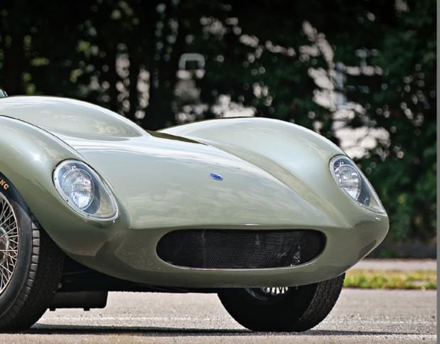
SPECIFICATIONS: Two-litre six-cylinder Bristol engine with three Solex carburettors, four-speed synchromesh gearbox, four-wheel disc brakes. Space frame steel tubing chassis with independent front suspension and De Dion rear. Aerodynamic alloy hand-formed body panelling. Wheelbase: 87"
